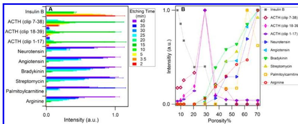
**Figure 3.** NIMS sensitivity study of nanostructured silicon substrates etched at 2 to 40 min using a variety of molecules ( $n = 20$ ). (A) Histogram of NIMS signals showing their intensity change by the substrates' etching time (the corresponding scatter plot is included in Supporting Information), (B) Scatter plot of NIMS signals by the substrates' porosity.
