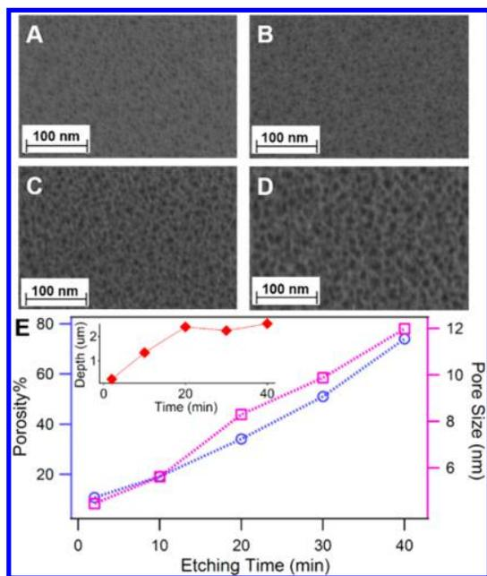
**Figure 1.** SEM images of etched silicon surfaces obtained at variable etching durations: (A) 2 mins; (B) 10 min; (C) 25 mins; (D) 40 min. (E) The correlations between surface morphologies of NIMS substrates and etching time: porosity in blue, pore size in purple. The inset shows the trend of etched depth with etching time.
