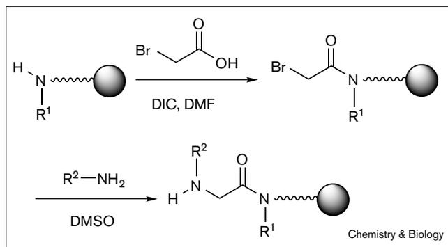
Scheme for synthesis of peptoids (poly *N*-substituted glycines) on the solid phase using the submonomer method. Each peptoid monomer is constructed on polymer beads by coupling bromoacetic acid to a secondary amine on the resin, followed by  $S_N2$  displacement of the bromide by a desired amine. DIC, diisopropylcarbodiimide; DMF, dimethylformamide; DMSO, dimethylsulfoxide.
